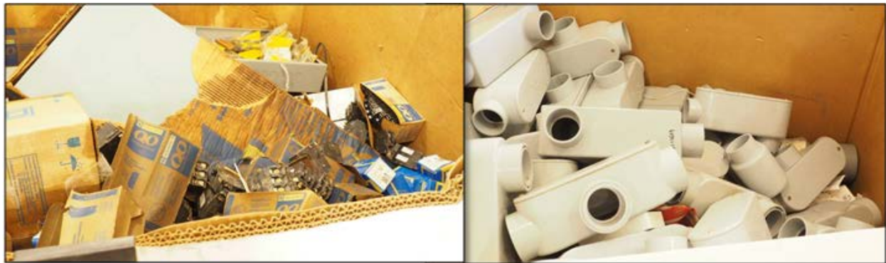
New Breakers (in manufacturer packaging) and Conduit Connections W/Cover slated for disposal – FSO Photos
